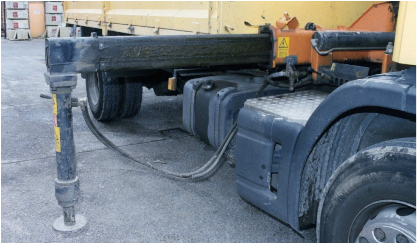
Close-up of the support leg that caused the accident
