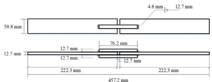
**Figure 3.** Transverse welded lap joints configuration
