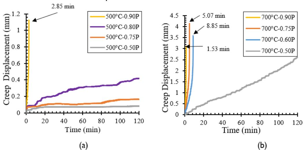
**Figure 11.** Effect of peak load ratio on thermal creep response of transverse welded lap joints at: (a) 500°C, (b) 700°C
