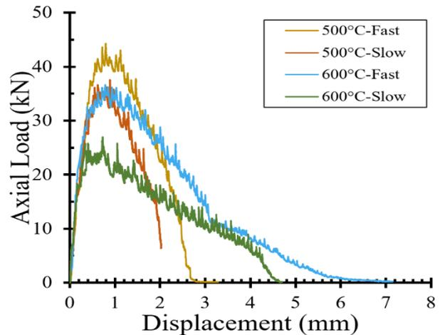
**Figure 8.** Results from tests performed at 500°C and 600°C under fast and slow loading rates
