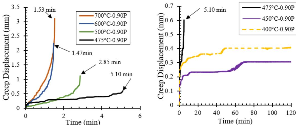
Figure 12. Effect of temperature on thermal creep response of transverse welded lap joints
