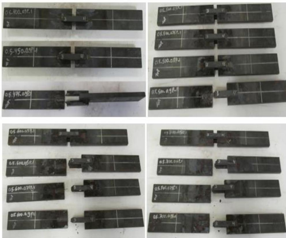
**Figure 9.** Failure mode for transverse welded lap joints for different temperature and load levels
