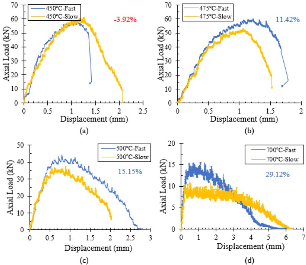
**Figure 7.** Effect of loading rate on the behaviour of transverse welded lap joints at: (a) 450°C, (b) 475°C, (c) 500°C, (d) 700°C
