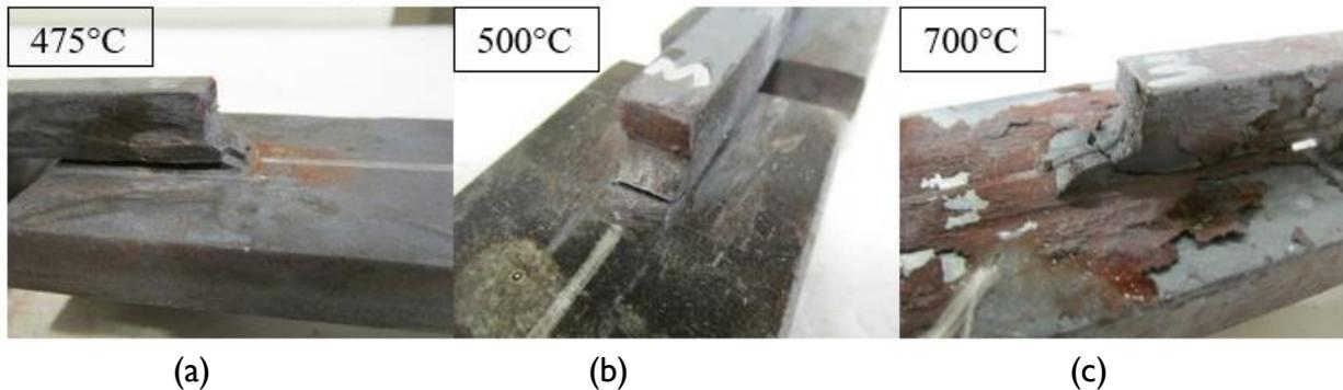
**Figure 10.** Creep fracture at the throat of the weld for transverse welded lap joints subjected to 0.90P at: (a) 475°C, (b) 500°C, (c) 700°C
