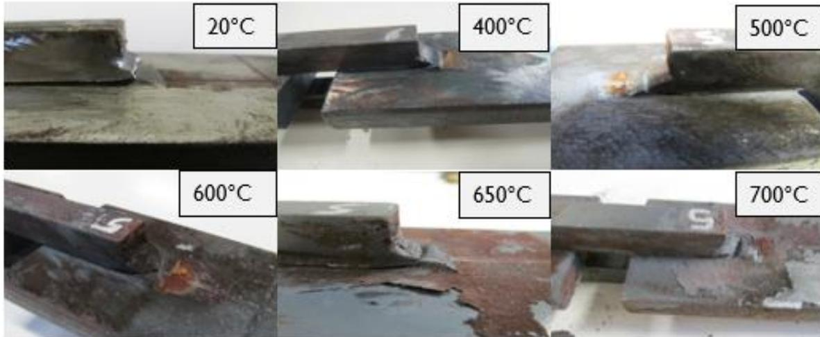
**Figure 6.** Failure modes for welded specimens subjected to ambient and different elevated temperatures
